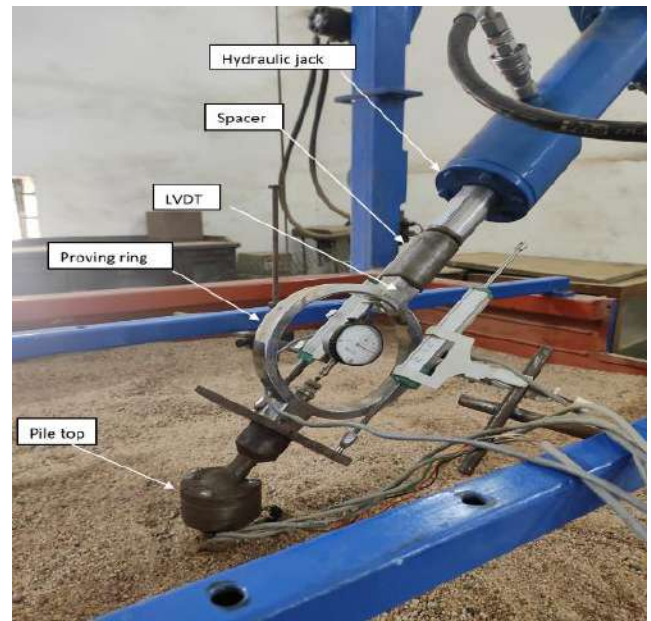
Load applied at 45^\circ with vertical
