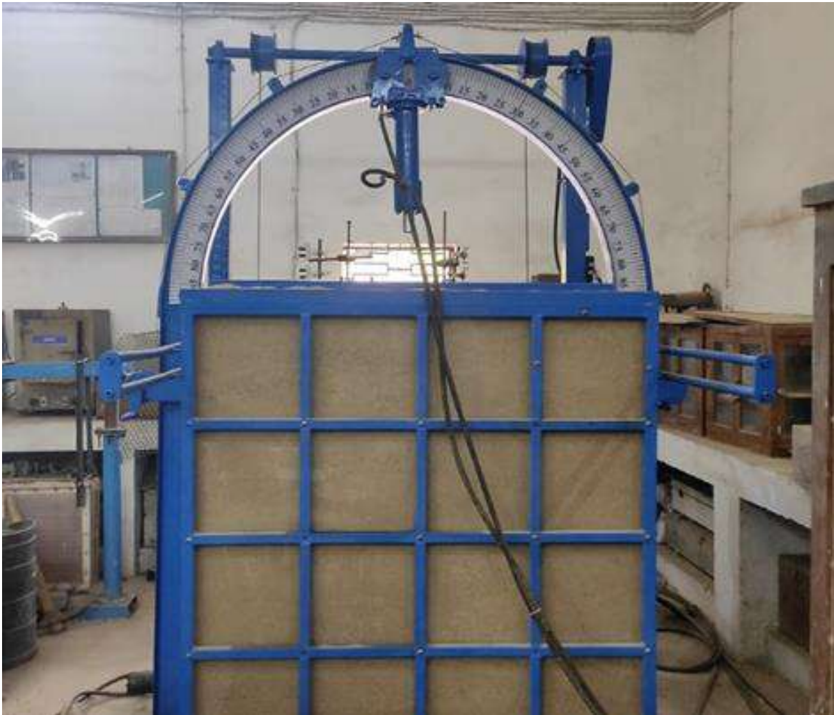
Fig. 3. Model Foundation test Set-up
