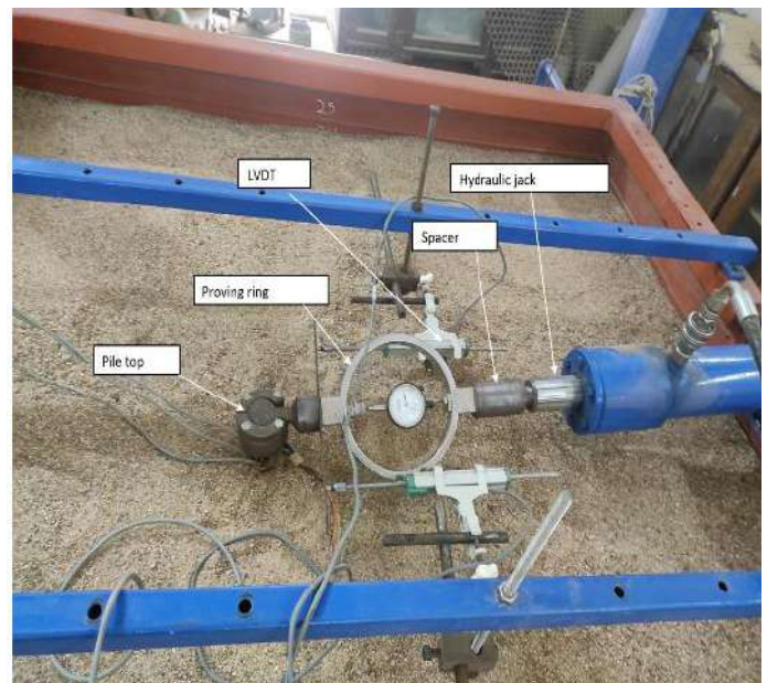
Load applied at 90^\circ with vertical
