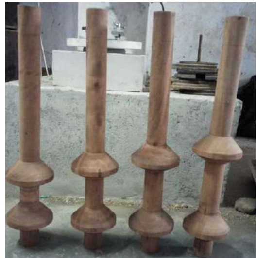
Fig. 2. Models of double under-reamed piles.
