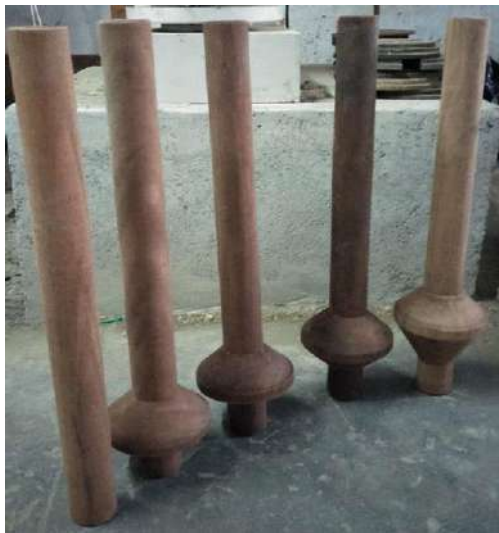
Fig. 1. Models of normal and single under-reamed piles.
