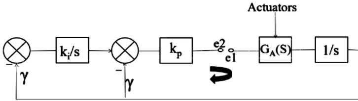
b) Corresponding Open Loop Controller of  $\gamma$  tracker
