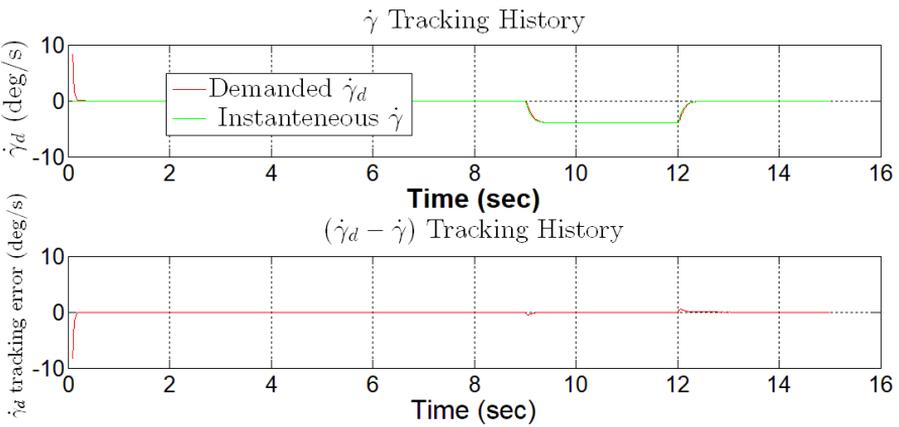
**Fig. 12.**  $\dot{\gamma}$  Tracking + Tracking Error
