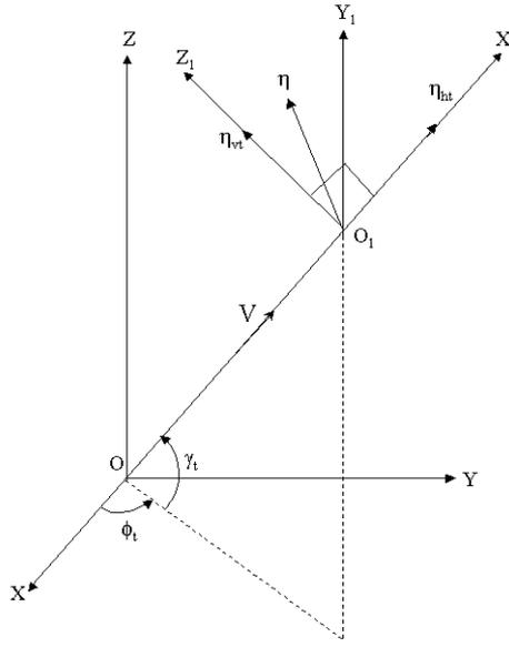
**Fig. 1.** Axes System for UAV Point mass model
