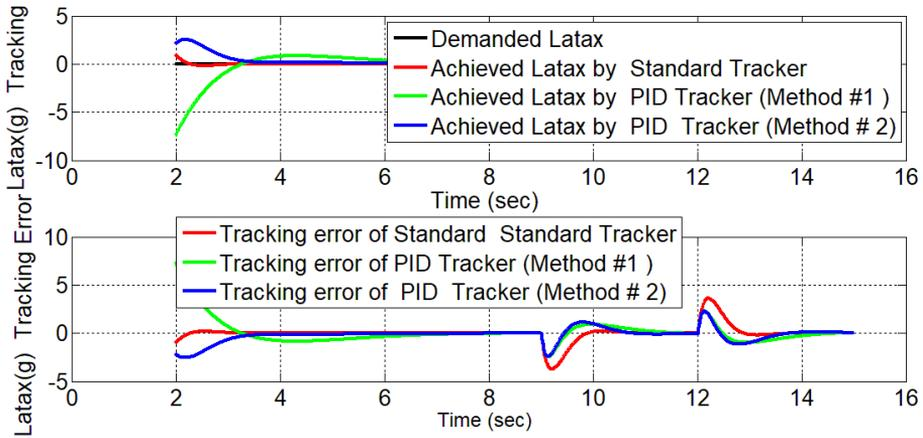
**Fig. 7.** Acceleration from Position Tracker (all cases)
