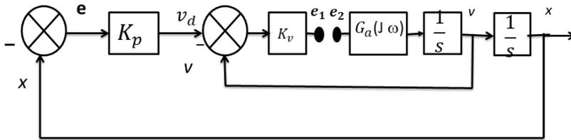
b) Corresponding open loop controller (position tracker)
