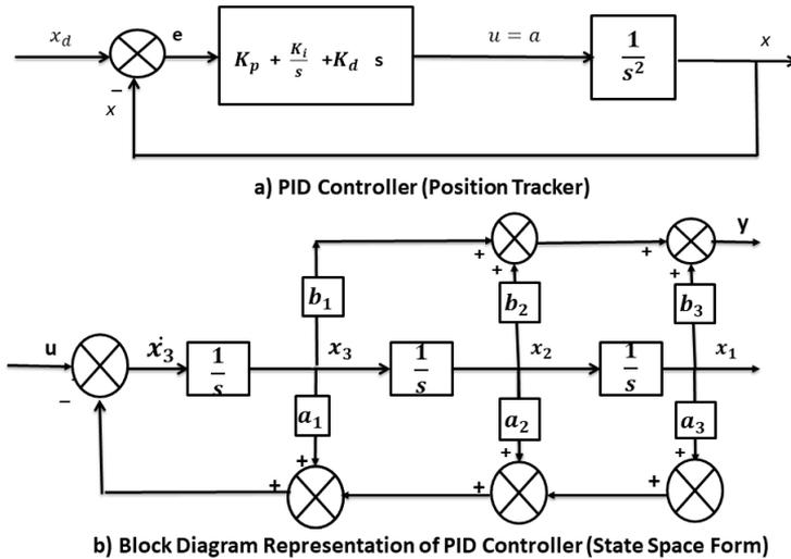
**Fig. 3.** Position Tracker (Closed + PID + Block Diagram)
