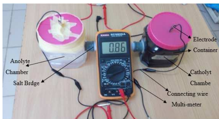
Fig. 1. A pilot system for a double chamber microbial fuel cell (MFC)
