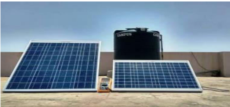
Fig. 3. 40W+75W Module at 3 pm in West Direction with 45° Angle at 21 st April
