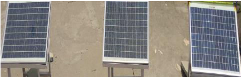
Fig. 1. On-field experimental set up at rooftop with three solar panels each of 40W placed on stands
